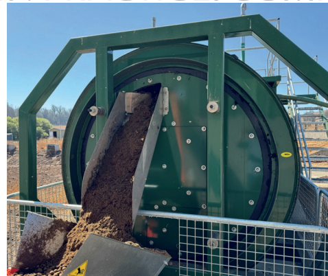
Correia Family Dairy uses a composter that turns biosolids into compost that is used as bedding resulting in the elimination of sand, financial savings, and healthier soils.
